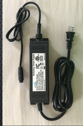
3 Amp Power Injection
